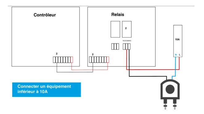
FOR SOME EQUIPMENT PUMPS, PAC, HEATING WITH A DRY CONTACT TYPE REMOTE CONTROL, YOU MAKE A RETURN TRIP BETWEEN THE COM / NO AND THIS CONTACT
