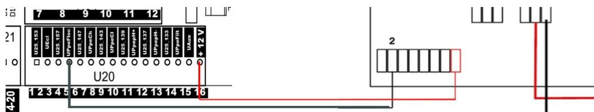
D'UN COTE NOUS AVONS LE CONTROLEUR AVEC SES 15 SORTIES DE PILOTAGE (POUR A2) ET L'ALIMENTATION COMMUNE DE 12V (A1)
